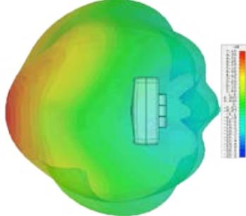
\*3D Patterns show realised gain both elements fed modelled in CST Microwave Studio without additional cable.
