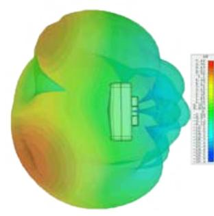
\*3D Patterns show realised gain both elements fed modelled in CST Microwave Studio without additional cable.
