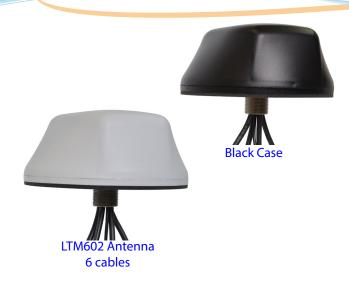
Mobile Mark's LTM601 Series Multiband Diversity/MIMO antenna contains six separate antenna elements, all in one compact antenna housing: two broadband LTE/Cellular antennas, three WiFi antennas, and one GPS antenna. The LTM601 covers Cellular LTE frequencies from 694-2170 MHz.
